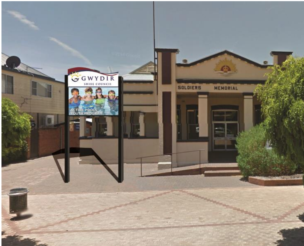
This mock-up shows an example of a single sided full colour P5 2,880 x 1,600mm LED sign with optional header board at the Maitland Street Bingara location
