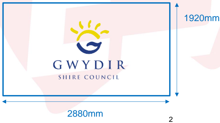
Video Board size 2880mm X 1920mm (Pitch 6mm)
