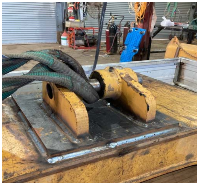
P1859 (Bingara grader) – repairs to ram mount on front blade
