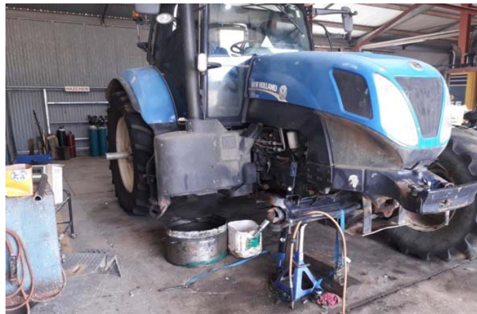
P1725 Tractor - wheel seals and bearing replaced in the Bingara workshop
