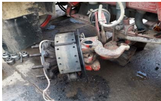
Replacement of king pin bushes on P1428 – gravel truck
