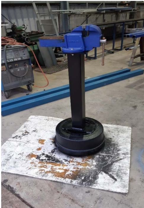
Vice stand has been fabricated for the Warialda landfill by a school based trainee
