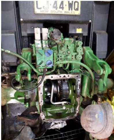
Plant 1866 hand brake and PTO repairs
