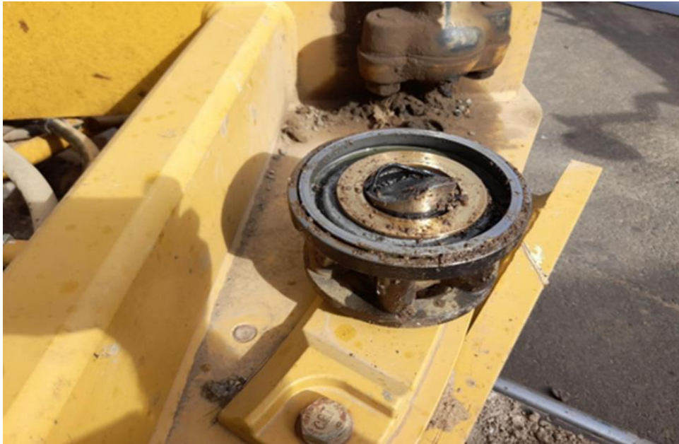
P1788 – repairs to (broken) shaft in turn circle
