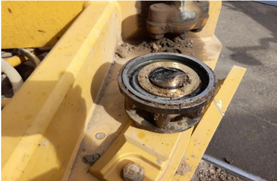
P1788 – repairs to (broken) shaft in turn circle
