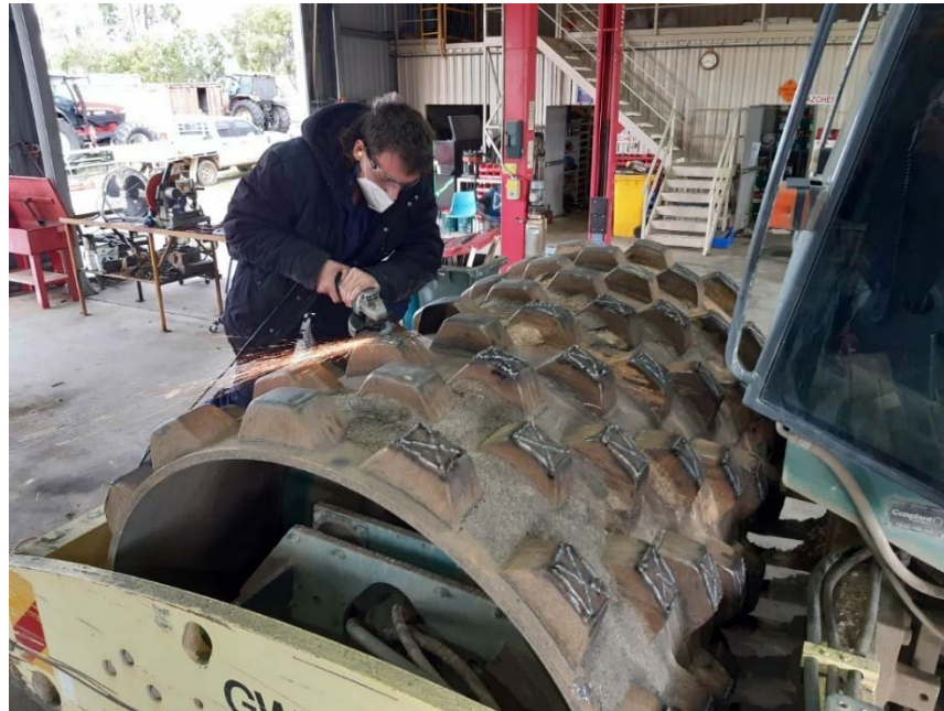
Trainee, Blake Mintoff hard facing the pads on P1474 Pad foot roller Warialda workshop
