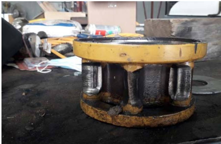
Replacement of worn-out turning circle in grader P1788
