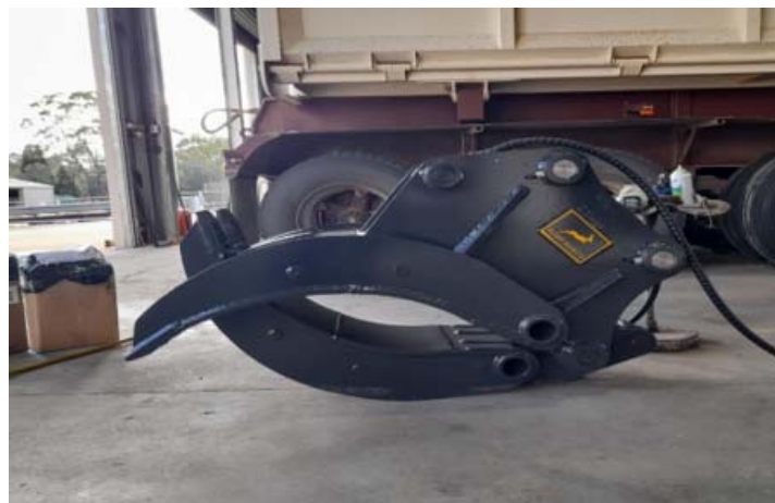
New 'grab' for 13T excavator P1986
