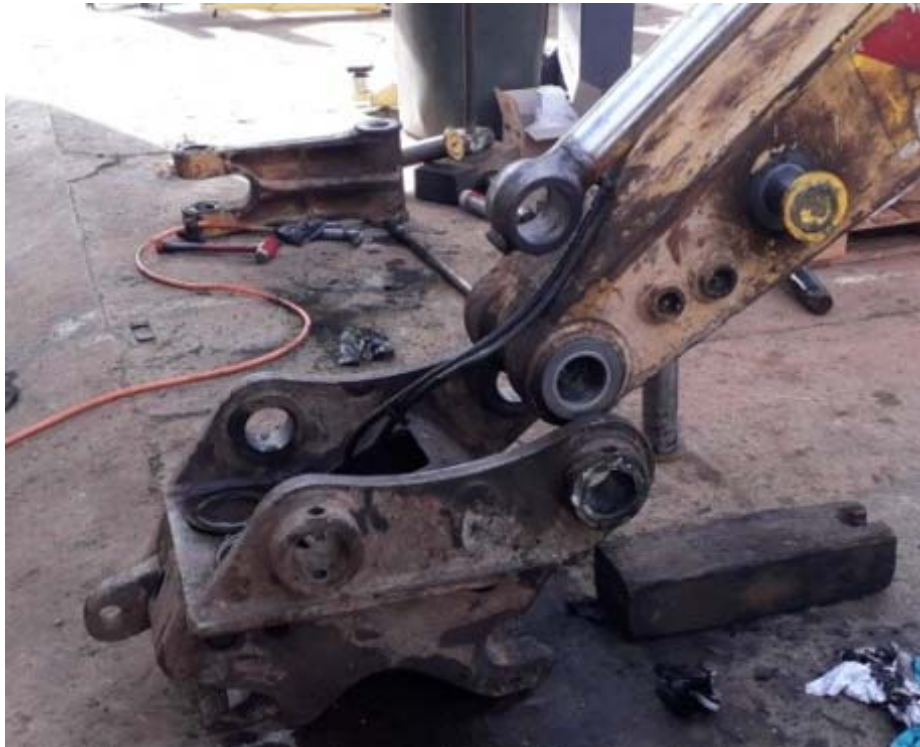
P1467 Komatsu excavator bush replacement (Bingara)
