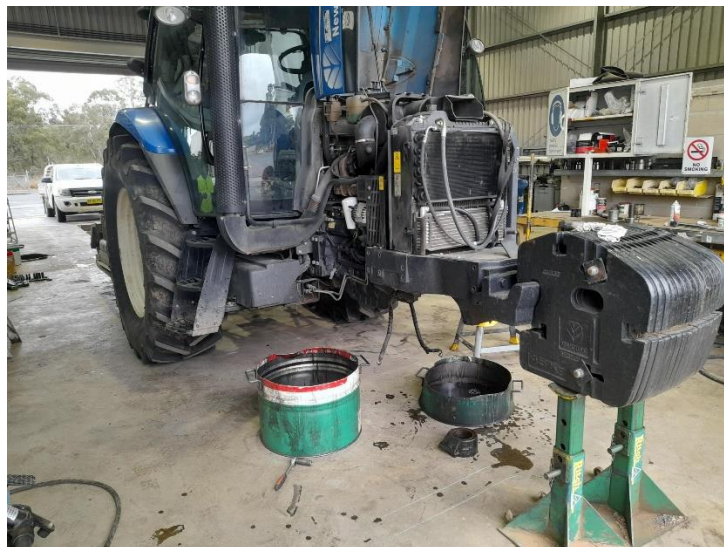
P1724 – Tractor differential repairs
