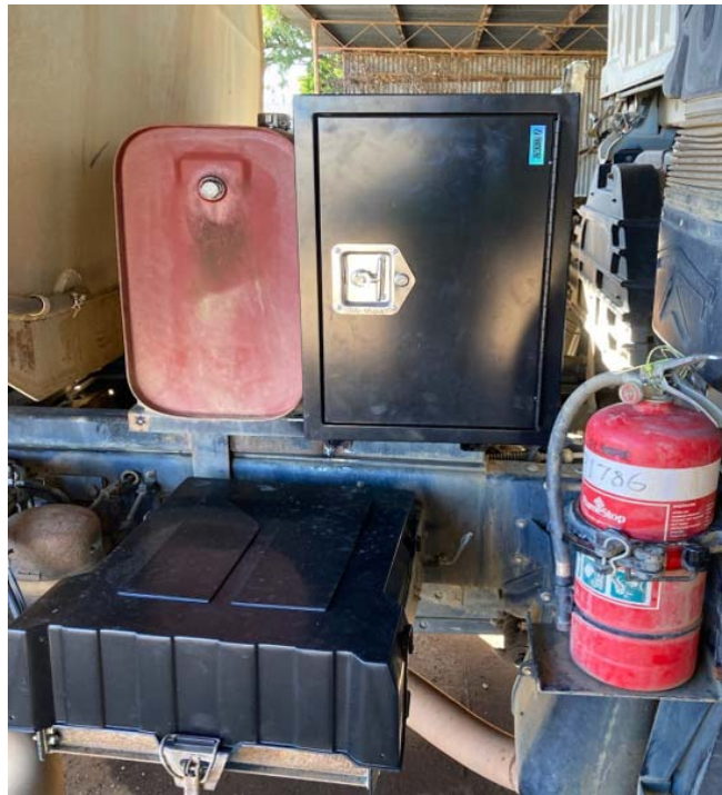
Watercart P1786 (Bingara) - relocation of toolbox and fire extinguisher
