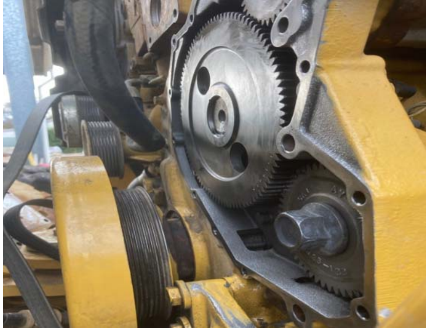
P1859 (Bingara grader) – repairs to timing, oil leak
