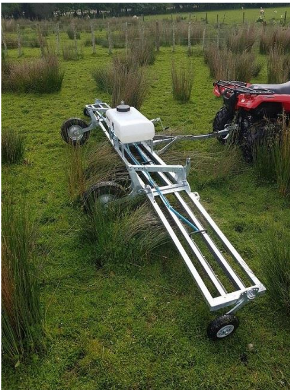
Figure 8: Commercially-made wick wiper designed for towing, with adjustable height.
