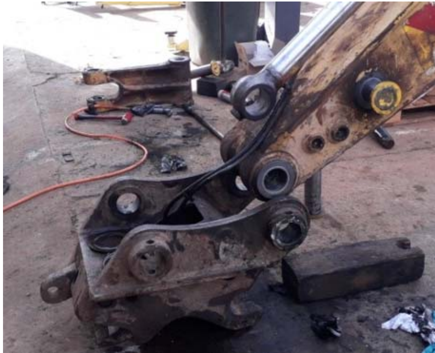
P1467 Komatsu excavator bush replacement (Bingara)
