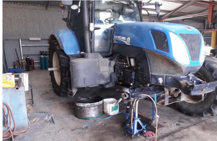
P1725 Tractor - wheel seals and bearing replaced in the Bingara workshop
