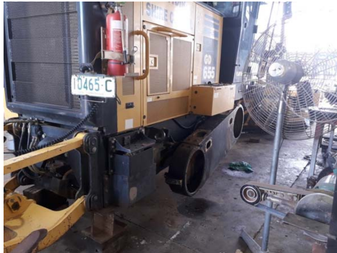
P1464 Grader - replacement of bearings seals and brake linings in the tandem drive
